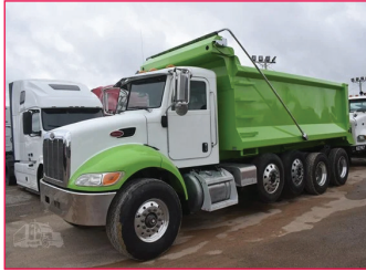
2012 PETERBILT 348 , Nice truck, runs perfect, clean truck, air gate, electric tarp, air seat, differential lock, double frame, dual steerable air lift axles, new bed, 504,804 miles, 370 HP. Stk. #12PETE504QUADDUMP ..... $65,000
