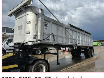
1984 CMC 35 FT Good trailer, good shape, electric tarp, air gate! Trailer is in good shape for age! *No title / bill of sale only! Aluminum composition, top hinge gate, all steel wheels, fixed tandem rear axle, center point suspension. Stk. #84CMC35DUMP ..... $10,000
