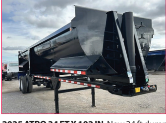
2025 ATRO 34 FT X 102 IN , New 34 ft dump trailer, high lift gate, built with AR hard ox steel, 13,337 empty weight, external cylinder/no doghouse for easier dumping capabilities, front ladder, led lights, *12% FET must be paid with purchase. Stk. #25ATRO397DUMP ..... $35,000
