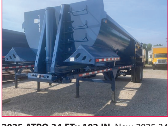
2025 ATRO 34 FT X 102 IN , New 2025 34 ft dump trailer, high lift gate, built with AR hard ox steel, 13,337 empty weight, extra cylinder / doghouse for easier dumping capabilities, front ladder, led lights, *12% FET must be paid with purchase. Stk. #25ATRO611DUMP ..... $35,000
