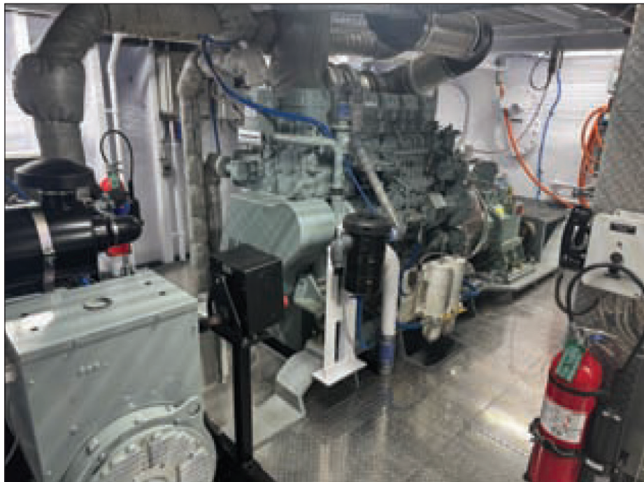
The mv. Sun Valley’s 1,600 hp, comes from a pair of Mitsubishi S6R2 Tier 3 engine supplies by Laborde Products.
