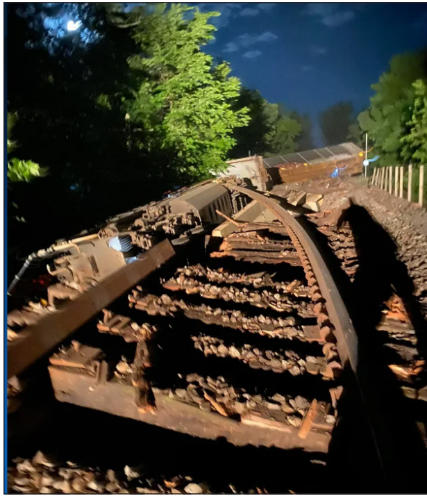
fallen onto the tracks. The collision caused 31 railcars to derail in various positions, including two locomotives.
