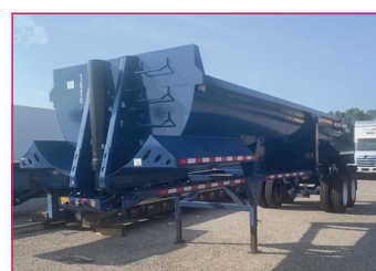
2025 ATRO , new 2025 34 ft dump trailer, high lift gate, built with air hard ox steel, 13,337 empty weight, external cylinder/ no doghouse for easier dumping capabilities, front ladder, led lights *12% fee must be paid with purchase! Stk. #25ATRO610DUMP..... $33,000
