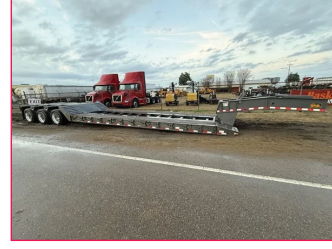
2026 WITZCO , New 52 ton detach lowboy trailers, 26 ft well, chain tie downs, polished alum wheels, air ride with dump valve and lift axle, adj ride height, out riggers, d-rings, Honda pony engine, chain/binder storage, factory warr. Stk. #26WIT045NGB52..... $68,000
