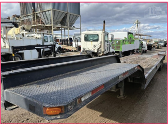
1981 CLARK 40 FT X 96 IN , Good trailer, good floor, good tires, flip ramps, Clark 25 ton Low Boy, 20 ft well length! Stk. #81CLARKLOW..... $10,000
