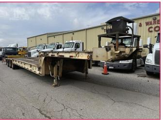
**2011 PITTS 50 FT X20 IN**, Good trailer, good tires, Pony engine, 32 ft. well, 50 ton payload capacity, fixed neck, air ride suspension, tri rear axles, gross vehicle weight 124,200 lb. Stk. #11PITT519TRILOW ..... \$30,000
