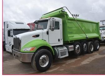
**2012 PETERBILT 348**, New truck, runs perfect, clean truck, air gate, electric tarp, air seat, differential lock, double fram, dual steerable air lift axles, new bed, 370 HP, 10 speed, walking beam, 17 ft body length. Stk. #12PETE504QUADDUMP ..... \$65,000
