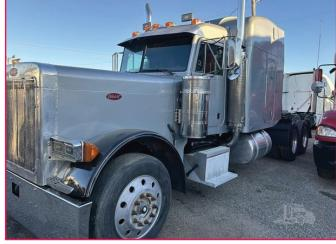
**1997 PETERBILT 379EXHD**, Good truck, runs excellent, dual exhaust, dual breathers, air seat, double bunk, differential lock, sliding 5th wheel, tilt/tele, dump valve, 10 speed, air ride suspension, manual Eaton-Fuller transmission. Stk. #97N14379 ..... \$30,000
