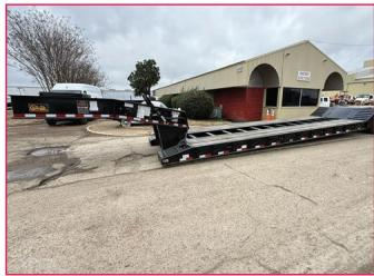
**2026 WITZCO CHALLENGER 51 FT x 102 IN**, New 52 ton detach lowboy trailer, air ride with dump valve and lift axle, adjustable ride height, out riggers, D-rings, Honda Pony engine, chain/binder storage, factory warranty. Stk. #26WITO26NGB52 ..... \$65,000
