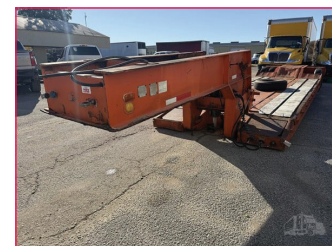
1973 ROGERS 42 FT , Nice trailer, good tires, well built, 20 ft well, requires wet kit to detach, ground bearing detach, 35 ton payload capacity, tie downs, wood floor, all steel wheels, tandem rear axles, 85,100 GVW. Stk. #73ROG18BLOW ..... $13,000
