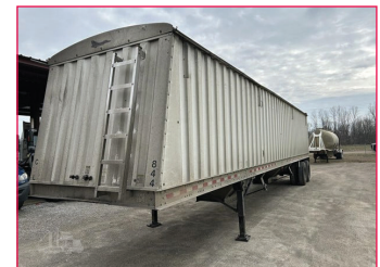
2015 JET 42 FT , Nice trailer, excellent shape, good roll tarp, good doors, nice wagon, two speed landing gear, two hoppers, front and rear ladders, air ride suspension, aluminum wheels. Stk. #15JET844HOPPER ..... $22,000
