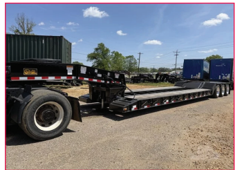
2027 WITZCO CHALLENGER 53FT X 102IN 52 TON , 24 ft well dove tail with ramps, chain with tie downs. chain/binder storage, 12% fet tax must be paid with purchase price. Stk. #27WIT004RG52DOVE..... $62,000
