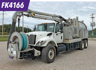
2008 International 7400 SFA 6x4 sewer jetter truck
